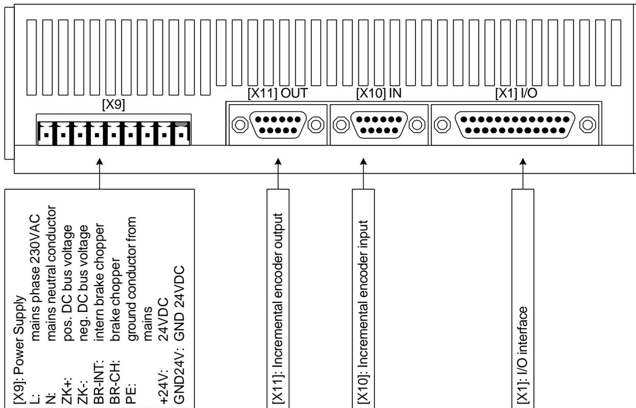
Figure 2: item servo positioning controller C 1-02: Top view
