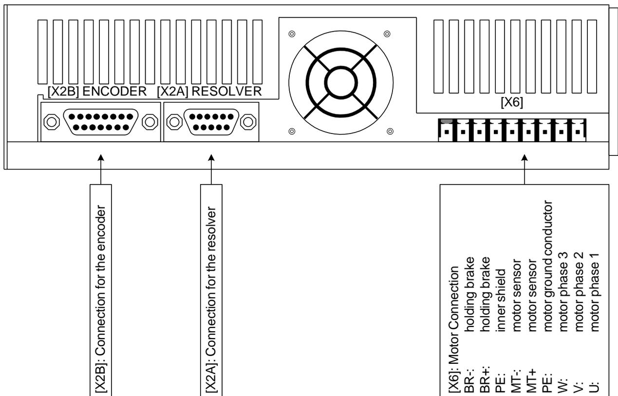
Figure 3: item servo positioning controller C 1-02: Bottom view
